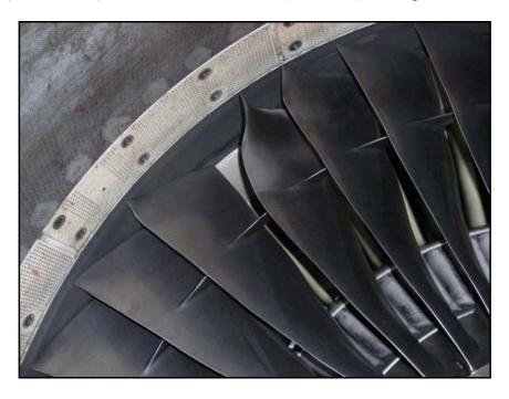
Photo No. 1: No. 1 Engine Fan Blade Damage
