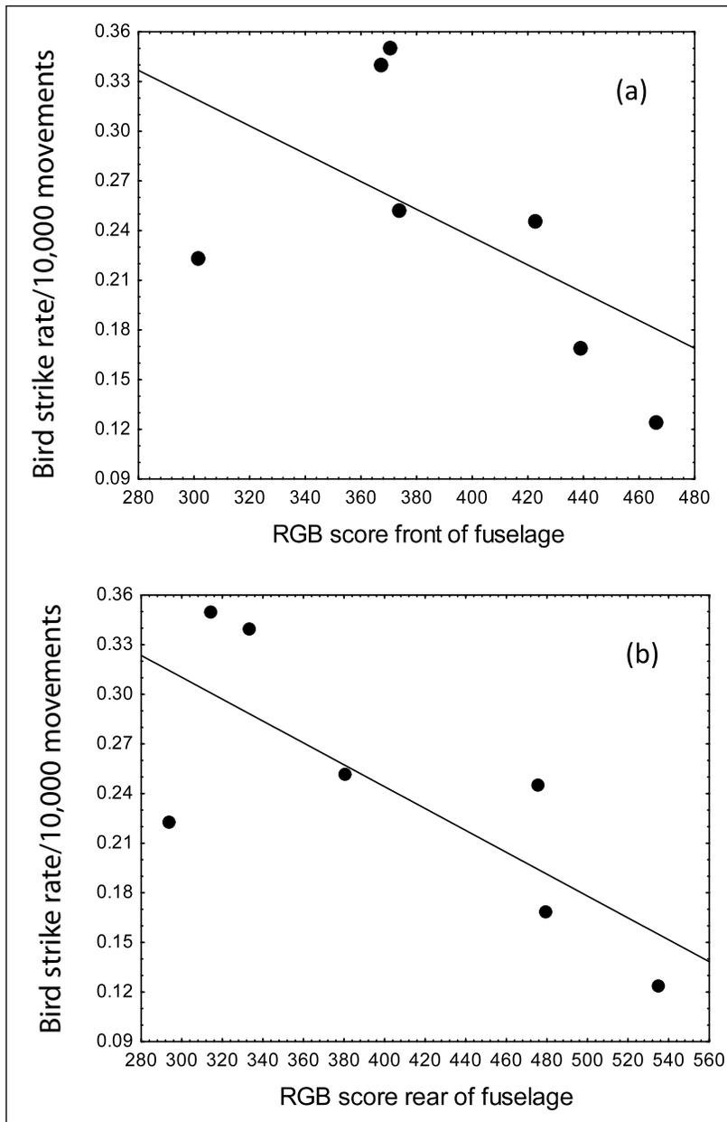
**Figure 2.** Relationship between bird-strike rates (estimated as number of bird–aircraft collisions per 10,000 departures or movements) and RGB (red, green, blue) score from the (1) front and (2) rear of the fuselage of Boeing 737 aircraft belonging to different airlines. Higher RGB values indicate brighter colors, whereas, lower RGB values indicate darker colors.
