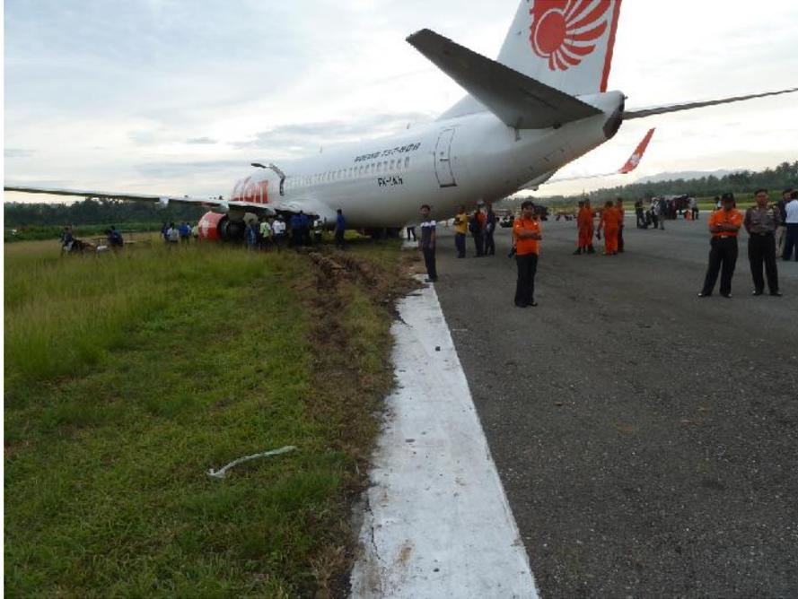
Figure 3. The aircraft out of the runway
