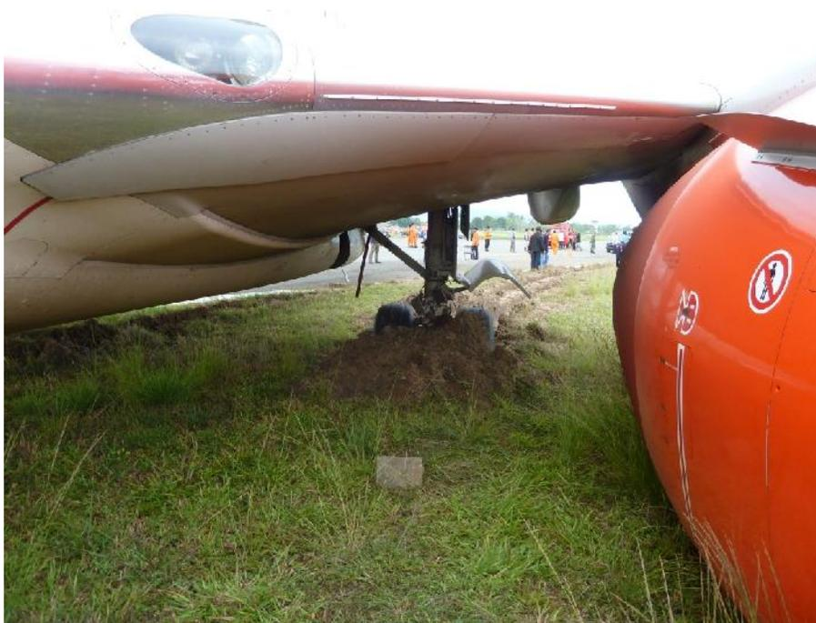
Figure 4. The aircraft wheels trapped on the shoulder
