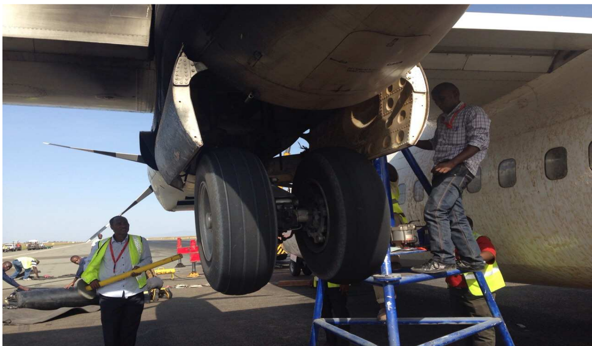
Figure 2: A photograph showing an engineer pulling the left MG down
