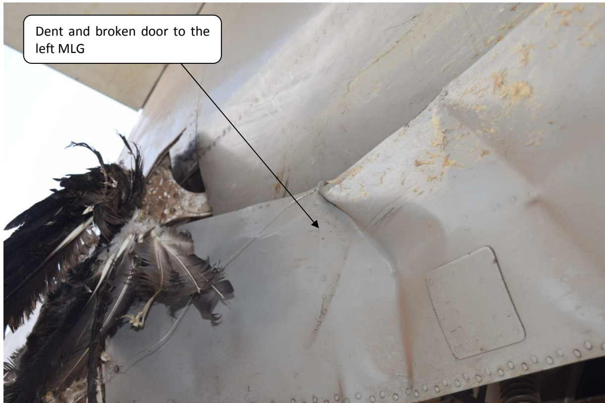
Figure 9: A photograph showing damage on the door to the left MLG
