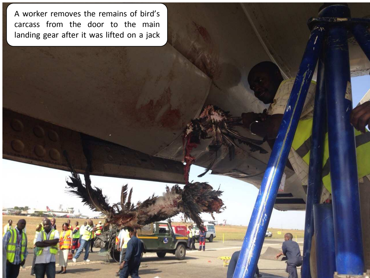
Figure 8: A photograph showing an engineer removing the bird's Caracas from the left MLG
